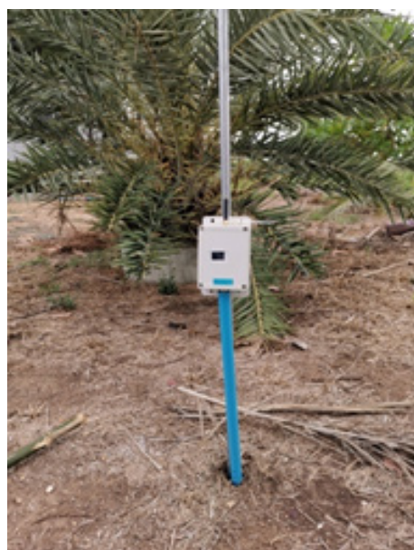
Figure 8. The soil sensor-node deployed in the crop area.
